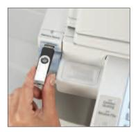
Load scanned documents onto portable media using Scan-to-Media capabilities with the **USB/SD card slot (optional)**. Print TIFF, PDF or JPEG files from the removable media.
